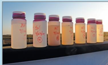
Left, a series of water samples retrieved near the mouth of the Tijuana River. Darker bottles contain more sediment, and samples like these allowed scientists to map patterns of sediment concentration along the coast. Far left, a dump truck adds sediment to the beach near the mouth of the Tijuana River as part of the demonstration project.
