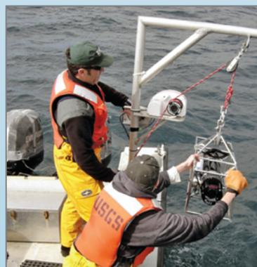
**Left, USGS scientists in Santa Cruz Harbor retrieve a grain-size-measuring instrument, which uses a laser to determine the size and concentration of sediment particles in the water column.**
